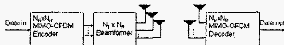
Fig. 1. MIMO-OFDM system with beamforming, where the number of transmit elements N_T = N_b , and the number of receive elements N_R = N_s .
