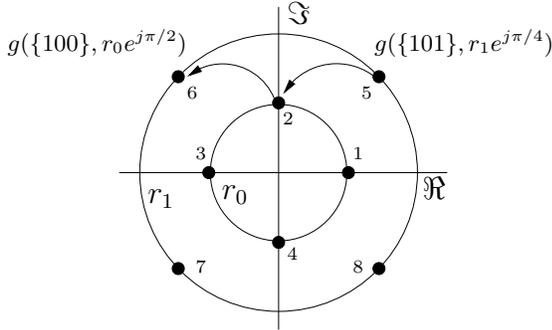
Figure 2: Differential 8-QAM signaling
